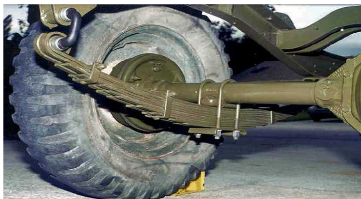
Fig 1: Leaf spring assembled at rear axle of automotive
